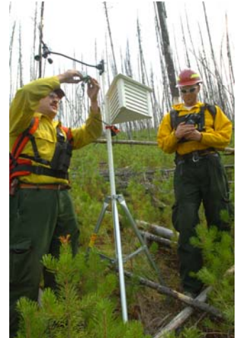
UM Fire Intelligence Module team members Carl Hartung and Saxon Holbrook set up a computerized network of weather sensors near a Montana Wildfire
