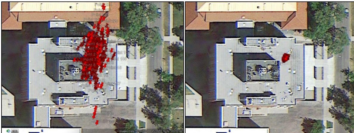
Figure 4. GPS-determined locations for stationary receiver (a) without external antenna and (b) with the external antenna.
