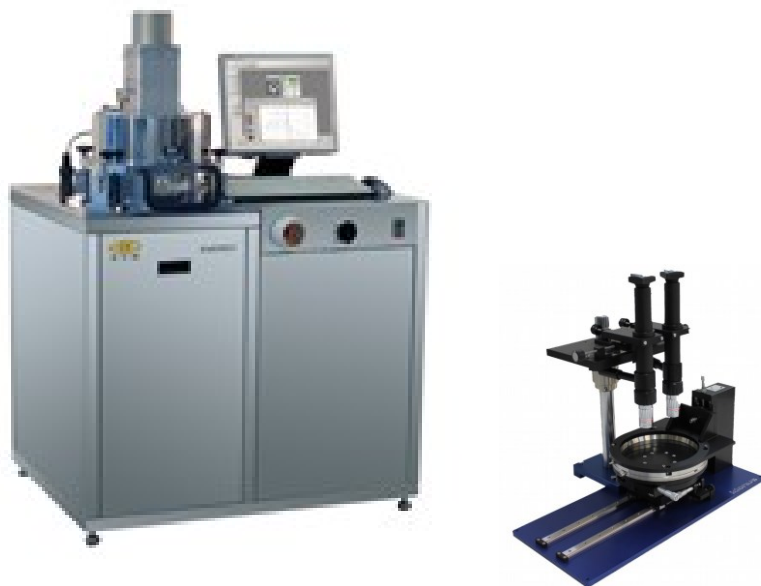
Figure 11: Desired EVG 501 bonder (left), a cheaper alternative from Idonus (right).
