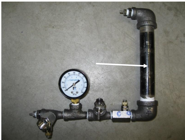
Figure 2. Steel reactor for analysis of TICP under flow conditions. Sand is packed in the straight 6” pipe portion of the reactor (arrow). Flow will be established in upflow direction and a pulsed injection strategy will be utilized initially, in which urea- and calcium-containing fluids are injected and then allowed to remain stagnant for ~24 hours.
