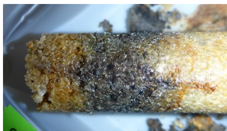
Figure 2. Thermally induced calcium carbonate precipitation was observed to bind together particles of sand after removal from the steel pipe batch reactor.
