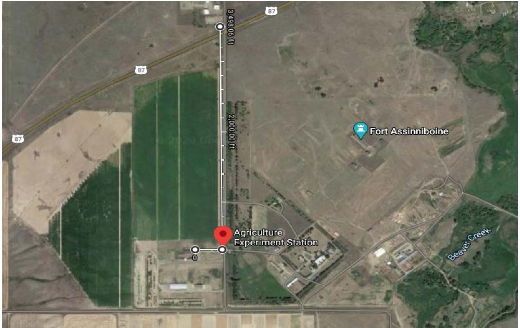
Figure 2. Proposed Fiber optic placement location from service area along Highway 87, then south along Assinniboine Rd. then West into the NARC office lab.
