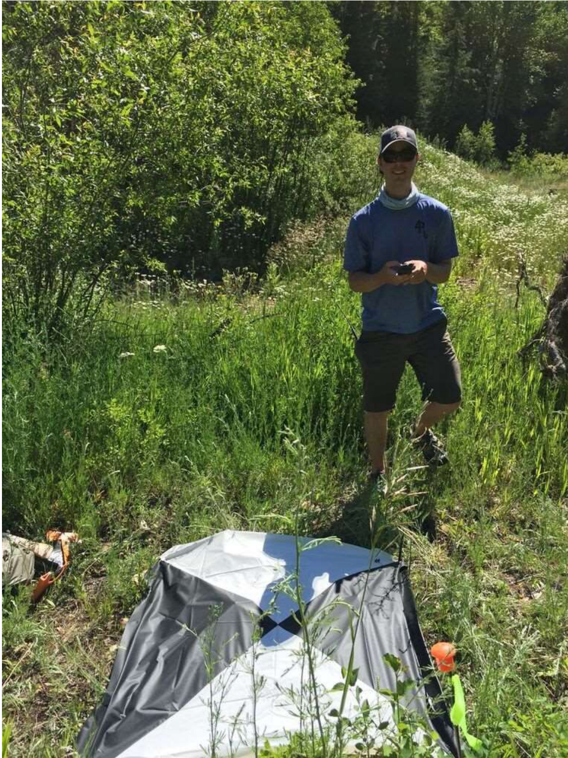
UM graduate student establishing ground control for drone data acquisition at the Ninemile Placer Restoration Project in the Ninemile Valley, MT.
